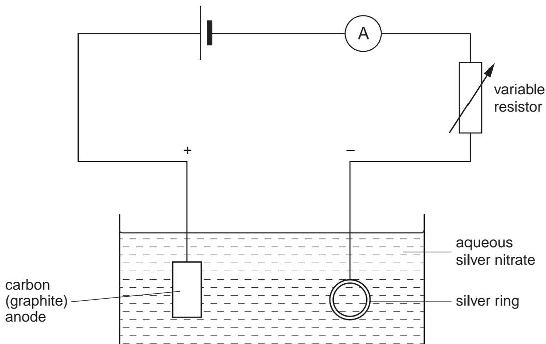
The ring, which was the cathode, was weighed before it was placed in the aqueous silver nitrate. The circuit was completed and a current of 1.0 A was allowed to flow.
